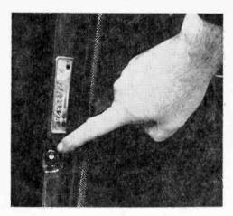
tesy light circuit. These switches are the self grounding type, always switching the ground lead of the courtesy lights: therefore, when you look at these switches you will see only *one* connecting wire. All other switches which may be added should be of the same type, self grounding, with their leads connected to the wiring of any of the original door switches. Additional switches for the hood, trunk or rear doors can be purchased from your car dealer at nominal cost.
