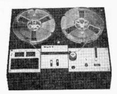
vide for both tape-in and tape-out signals at a single DIN jack, you can connect the Sony to this jack through a single multi-conductor cable. Otherwise, you use the standard phono-type line-in and line-out jacks. The microphone jacks, which are mounted along with the L- and R-record volume controls and the record interlock under a hinged cover on top of the deck, are the *mini* type. The TC-350 does not accommodate the standard phone-type microphone plug.
