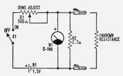
Fig. 3. Schematic diagram of Mini-Ohmer has only one difference from circuit in Fig. 2—R2 in shunt with meter. Meter indicates IR drop across R2 and unknown.
