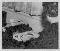
Stencil is ideally cut on a typewriter, but a ball pen or a metal stylus can also be used. Clean, clear stencil works best. Type carefully!
