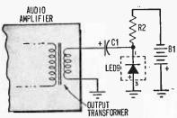
Fig. 2. Simplified schematic of output circuit used to modulate gallium-arsenide diode.
