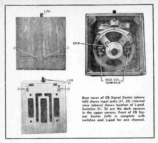
While a metal enclosure might look more pro, keep in mind that a wood baffle produces a superior sound, with none of the metallic "ring" common to metal enclosures (you'll be surprised how good your transceiver sounds when you get the speaker out of the metal coffin).
