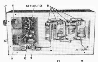
Fig. 10. Completely wired transmitter (above) only needs to have mirror and GaAs diode mounted at one end.
