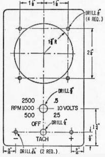
Layout of front panel of Tach Stretcher accommodates the Knight 0-50 microammeter.
