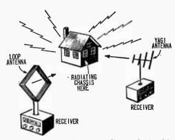
Some sources of ITV must be tracked with direction-finding techniques. Loop and Yagi antennas are easily made and should be tuned to the interference frequency.
