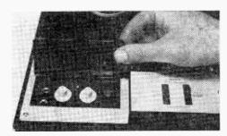
Snap-open door on top left conceals the 350's mike jacks and record level controls. Two mode switches are directly below heel of hand.
