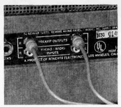
Outputs from master unit should ideally come from preamps. This way, any distortion in unit's power amps can be bypassed.
