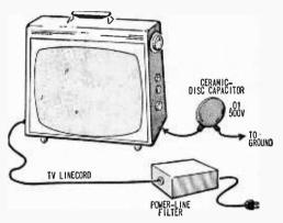
Metal-cabinet TV sets are easy to ground but plastic and wooden cabinets do not act as shielding unless lined with metal foil.
