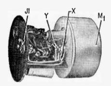
Internal view of Knight tachometer shows location of J1 and added solder terminal.
