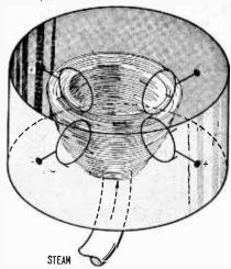
Fig. 7. With charged grids mounted in a circle, steam (injected at bottom) formed a rapidly turning tornado-like vortex in test chamber.
