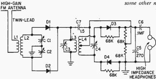
You might try the circuit shown in the diagram. It uses four diodes capable of VHF operation. The first stage is a frequency doubler. It doubles the FM signal frequency and the FM deviation so that the detector will recover more audio. L2 is tuned by C1-C2 to the FM band. L3-C3 and L4-C4 are tuned to twice the FM-band frequency. It *might* work if the signals are really strong.
