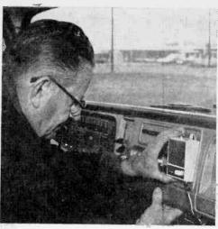
Master intercom unit is mounted on dash of pickup truck. Make sure wiring isn't dangling—tape it securely to bracket behind dash.
