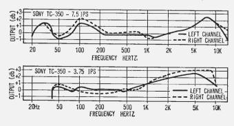
Curves show overall record/play response at both 3 \(^3\)/2-and 7 \(^1\)/2-ips speeds for Sony 350 tape recorder (the identical tape deck, mounted in a carrying case for portable use, is also available as the Model 350C). Note that response actually extends to a low 20 Hz at the faster 7 \(^1\)/2-ips speed.
