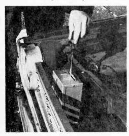
Once Auto Siren Sentry is attached to the body, leads to switches can be connected. Protect leads from accidental breakage and possible tampering through grill openings.
