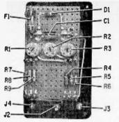
Internal view of the Tach Stretcher shows mounting of components on the circuit board. R1, R2 and R3 are calibration controls.
