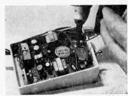
It takes a steady hand and a small soldering iron tip to make necessary speaker connections.
