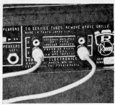
Tape recorders vary in way their inputs are labeled, but it's best to select high-level, low-impedance inputs in the slave.
