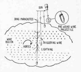
Fig. 11. Wires might be launched through charged area using coiled-wire projectile.
