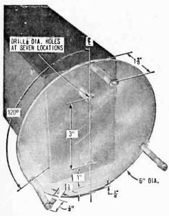
Fig. 7. Dimensions of mirror mount are given above. Disc can be cut from wood, plastic or fiber as long as material is rigid enough to hold mirror in place and will not be affected by variations in temperature or humidity.
