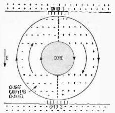
Fig. 5. A charge-carrying channel in the vortex moves positive and negative charges in opposite directions between charged cloud areas. Grids supply charge in laboratory.
