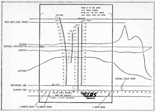
Each Air-India Boeing 707 has a Lockheed Aircraft Service 109-C flight recorder mounted inside left-hand wheel well (left), close to center of gravity. The crash-proof spherical container has been tested to withstand temperatures up to 2,000°F and impact of 500g. Traces on tape (above) can be read easily with transparent scale placed over recorded tape.
