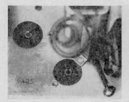
Finished result shows 6AQ5 tube designation "engraved" on the chassis. Kit is not suitable for use with anodized, coated metals.
