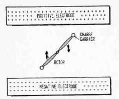
Fig. 2. Diagram of electrostatic motor shows how rotary motion is developed in vortex by effect of accumulated high-voltage charge.
